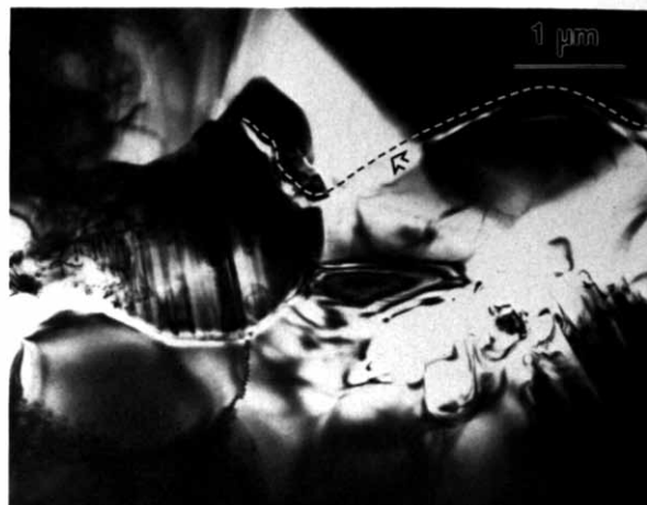
Fig. 9. TEM evidence for interaction of intergranular microcracks (arrow) with ZrO_2 particles in AT80.
